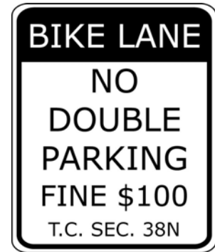
This sign may be used to discourage motorists from parking in bike lanes.
