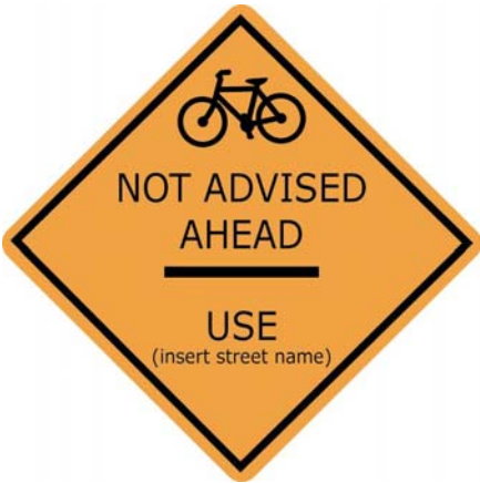
This sign may be used to indicate an alternative route for bicyclists.
