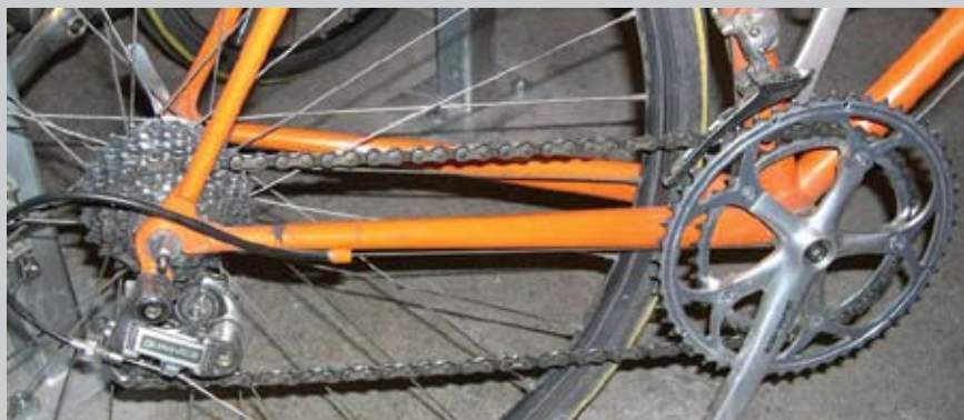
Side view of a bicycle drive-train: rear gear cogs; rear derailleur, chain, front derailleur, front chain rings and pedal cranks.
