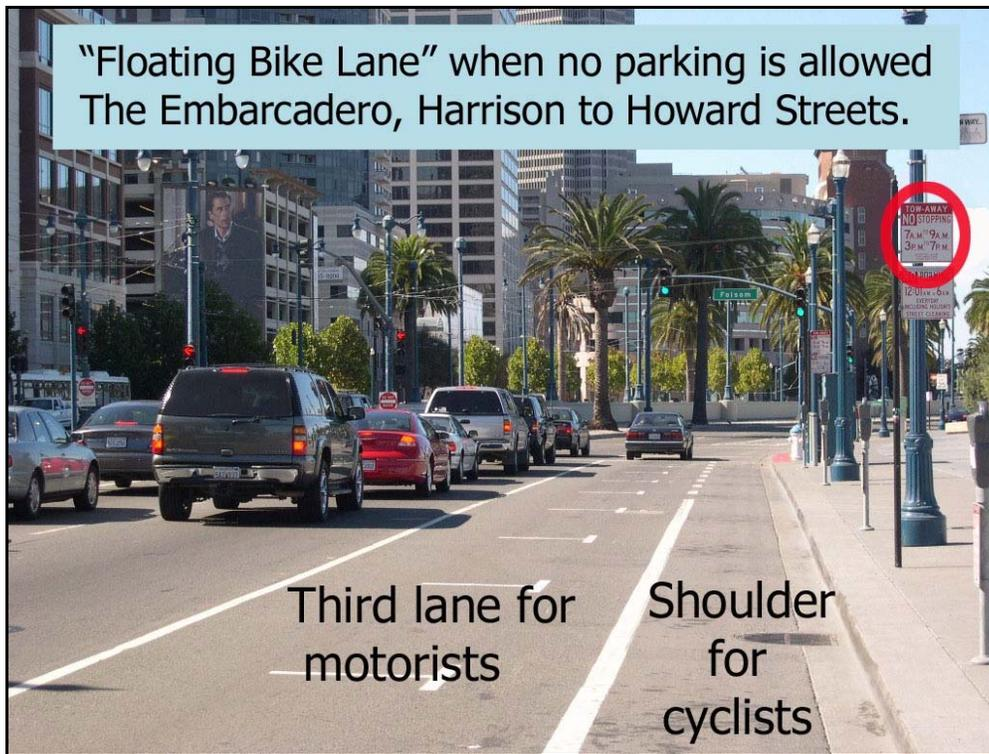
Figure 2. “Floating Bike Lane” with Part-Time Parking when Parking is Not Allowed
