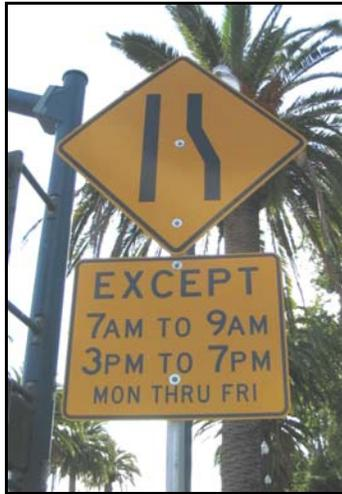
Figure 4. Merge Sign at Beginning of “Floating Bike Lane” Treatment where Three Full-Time Lanes Approach Two Full-Time Lanes and One Part-Time Lane
