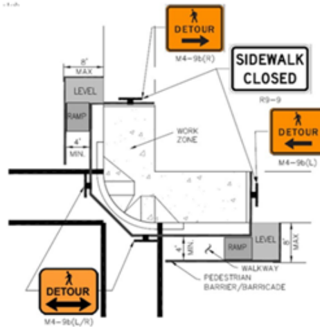
Figure 5.1b Pedestrian Detour at Intersection Corner (Non-Work Hours)
