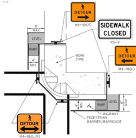
Figure 5.1b Pedestrian Detour at Intersection Corner (Non-Work Hours)
