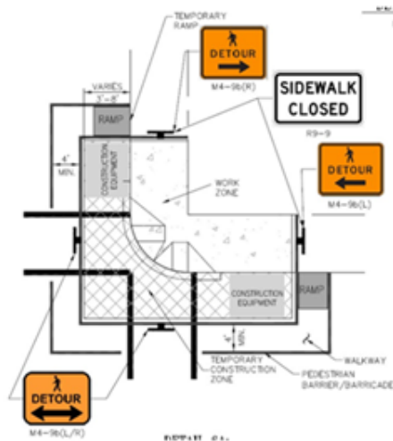
Figure 5.1a Pedestrian Detour at Intersection Corner (Work Hours)
