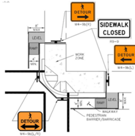
Figure 5.1b Pedestrian Detour at Intersection Corner (Non-Work Hours)
