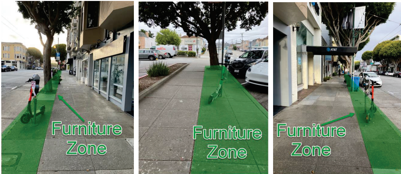
Figure 2b. - Properly Parked in the Furniture Zone - The images below are examples of devices properly parked in the furniture zone. In areas where there are no racks available, devices may be locked to meters and sign poles help keep devices from being knocked over or moved into the accessible path of travel.
