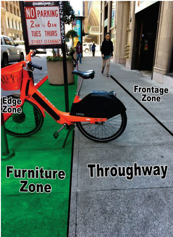
Figure 1c. – Additional Furnishing Zone illustration – This device also extends outside of the furnishing zone, impeding the throughway.
