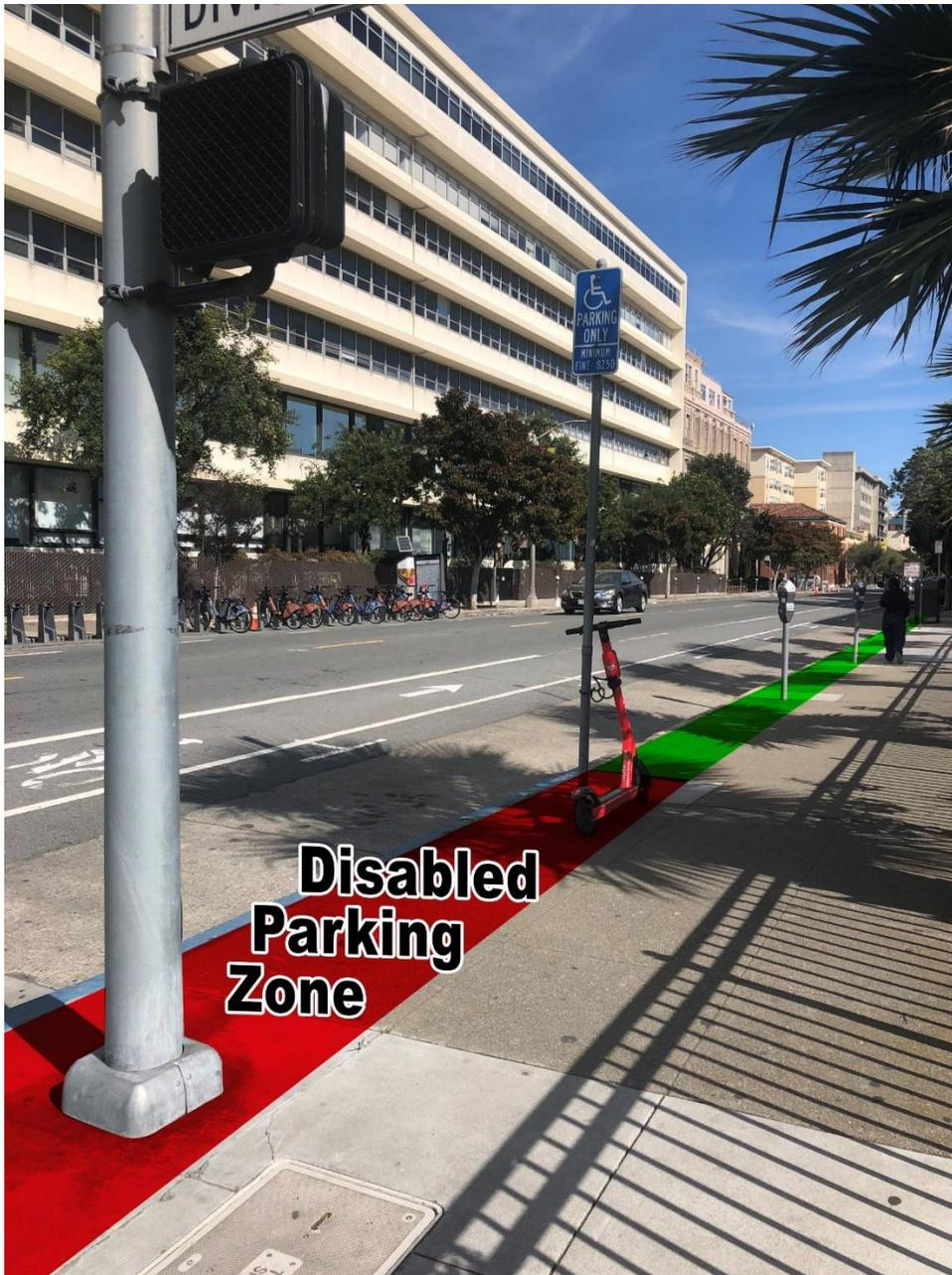
**Figure 6 – Footprint of the Rack Illustration** – The devices shaded in green depict devices parked within the footprint of the rack. The device shaded in red depicts a device parked outside of the footprint, which is considered improper. By parking outside of the rack footprint, devices impede the path of travel.
