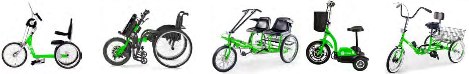
(L-R) Seated Handcycle, Manual wheelchair power adapter, Dual seated pedal powered three-wheeler, Seated, three-wheeled electric scooter, Compact balance stability tricycle
