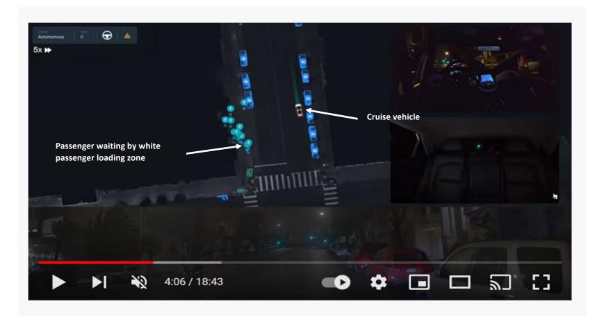
Below is an example where the Cruise vehicle stops in the travel lane to drop off the passenger. Curb space is available both immediately in advance of and immediately beyond the location where the vehicle stops in the travel lane to unload a passenger.
