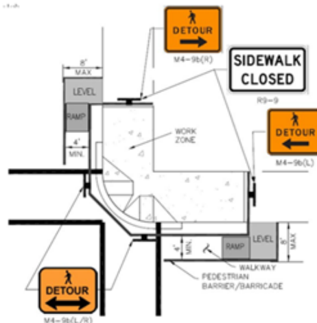
Figure 5.1b Pedestrian Detour at Intersection Corner (Non-Work Hours)
