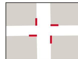
Where geometrically feasible, intersection daylighting is proposed at all intersections along the Neighborway. Existing daylighting will be refreshed.
