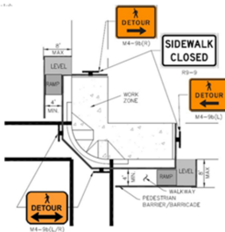
Figure 5.1b Pedestrian Detour at Intersection Corner (Non-Work Hours)
