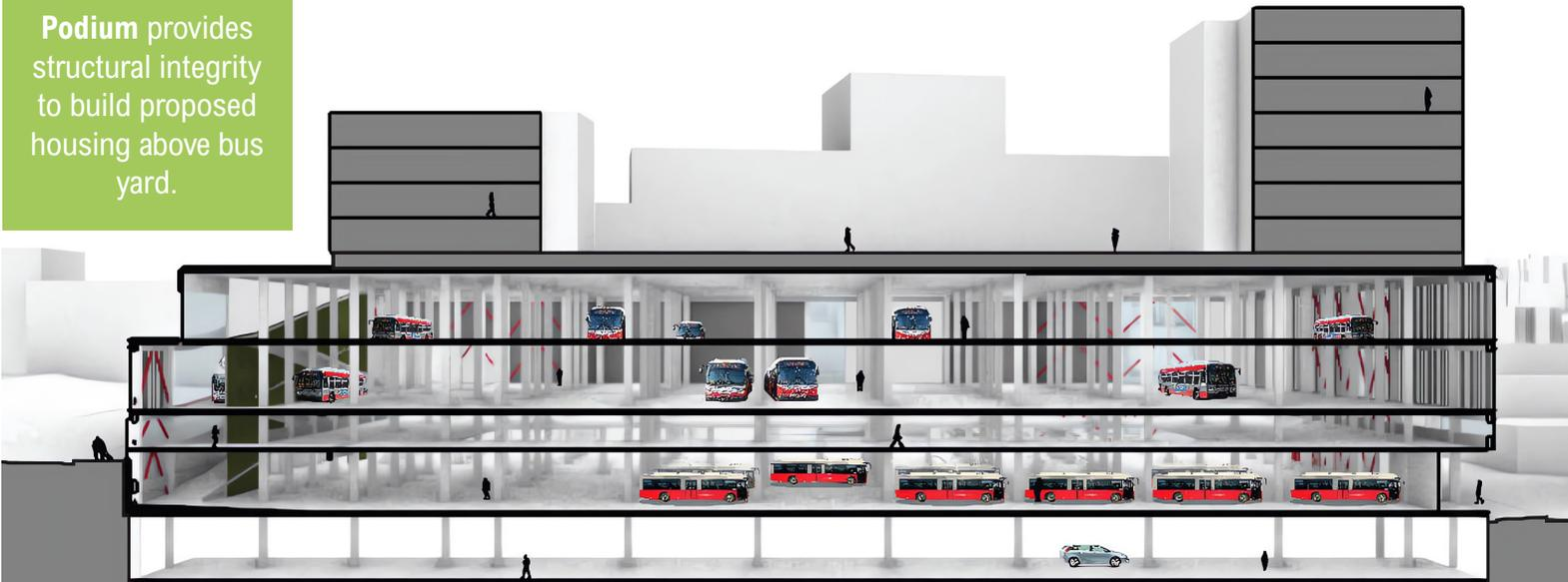
**Enclosed and Centralized Maintenance** activities on ground floor to insulate noise within building.
