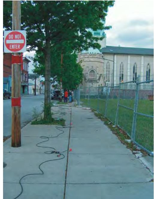
**Microtremor Measurements along Sidewalk**
