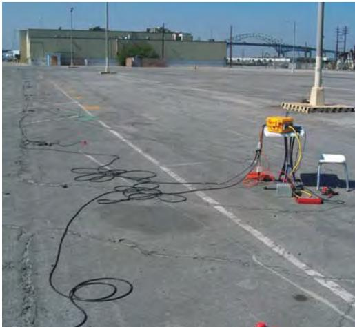
**Refraction Microtremor Array Layout**
