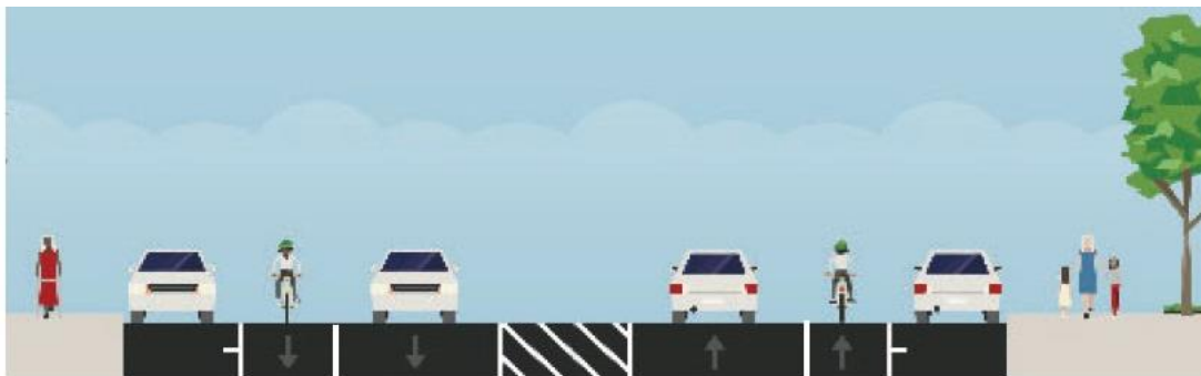
Figure 2: Existing typical mid-block cross-section of Winston Drive
