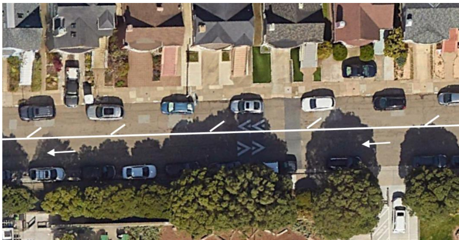
Figure 5 - Illustration of Lenox Way edgeline to visually narrow street and provide room to back out of driveways
