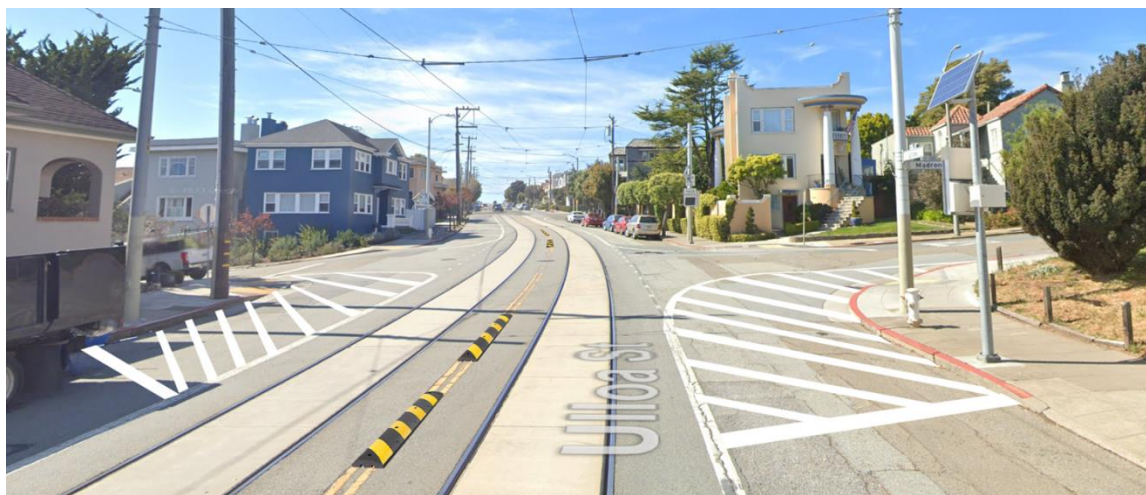
Figure 3 – Conceptual illustration of Ulloa traffic calming proposals: painted roadway markings would complement a hardened centerline to physically and visually shrink the roadway.
