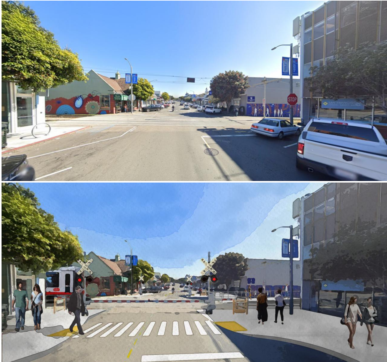
Figure 14: Crossing gates may help improve the safety of transit signal pre-emption. Particularly, at unusual intersections where cars may be surprised by a stop light. A few examples are where the M Ocean View crosses Eucalyptus Drive, Ocean Avenue and 19th Avenue at Rossmoor Drive. This image is an illustration of possible upgrades at Ocean Avenue (existing conditions at top), including crossing gates.
