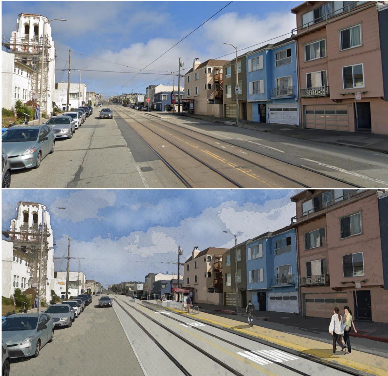
Figure 18: Photo illustration of possible upgrades to an example N Judah stop to provide level boarding
