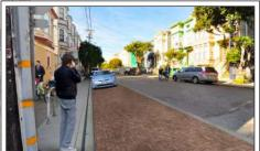
PERMEABLE PAVEMENT enables stormwater to soak through the roadway and into the ground, rather than rapidly flush into the sewer system.
