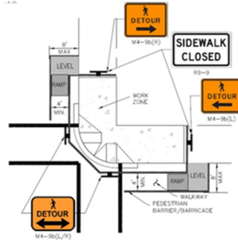
Figure 5.1b Pedestrian Detour at Intersection Corner (Non-Work Hours)
