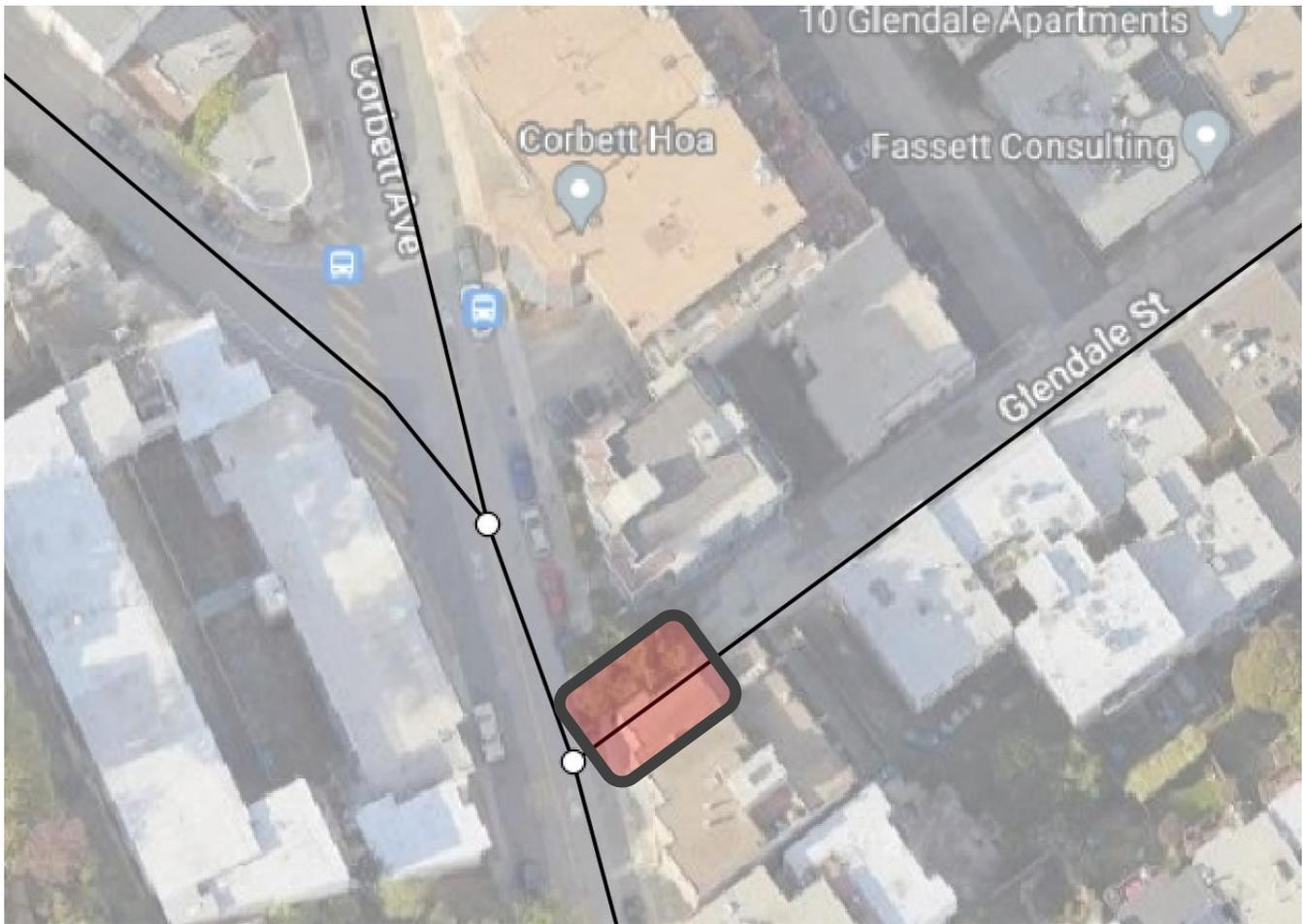
Figure 5: Example where network GIS data incorrectly represent two intersecting streets.
