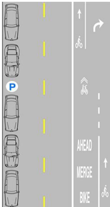
Fig. 9.1 Illustration of elements for shifting a bike lane to the left side of right turning vehicles
