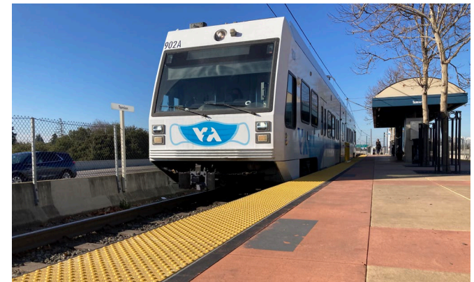
Example of low-floor station platform in San Jose, VTA
