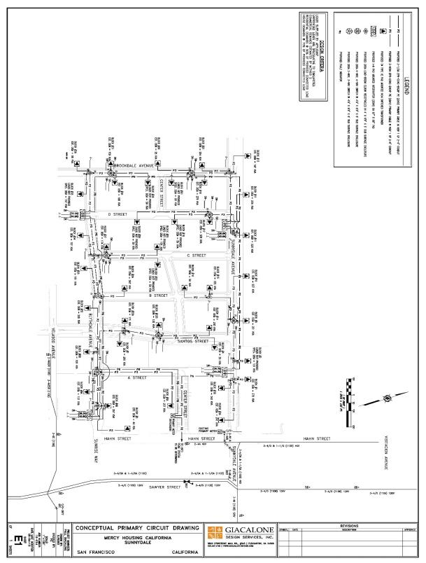
Figure 14.4 Conceptual Joint Trench Plan
