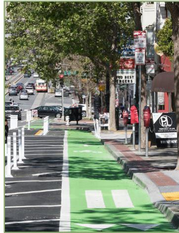
Green pavement is used in a variety of ways across San Francisco, usually to highlight the presence of bikes. It can be used to highlight bike lanes, striped through conflict points and intersections, or used to improve the visibility of sharrows.
