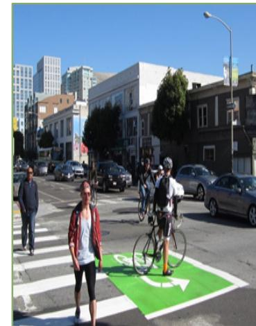
A marked area on the far side of a crosswalk to facilitate safer left turns for bicyclists. It addresses turning conflicts, visibility issues, and prioritizes bicyclists' movement at the intersection. Works especially well for turning movements to, or from, a protected bikeway.
