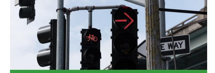
On average, bikes comply with the traffic signal indications 86 percent of the time at the two observed locations with separated bike signals.
