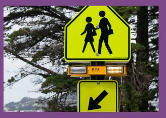
Rectangular Rapid Flashing Beacons are useractuated amber LEDs used at unsignalized intersections or mid-block crosswalks. In San Francisco, most RRFB's can be activated manually when pedestrians push a button. This evaluation collected data at two locations before and after the installation of RRFBs. We will be evaluating at least four other locations in 2019 to better understand efficacy of this tool.
