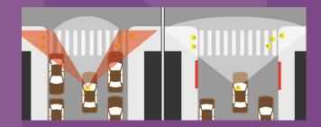
Daylighting removes visual barriers within a minimum of ten feet of a crosswalk or intersection to maintain sightlines, and is a straightforward improvement that makes everyone on the street easier to see at intersections.
