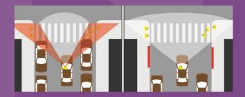
Daylighting removes visual barriers within a minimum of ten feet of a crosswalk or intersection to improve sight-lines, and is a straightforward improvement that makes everyone easier to see at intersections. Daylighting, or red zones at intersections, improves sight-lines and visibility between drivers and people crossing the streets in the Tenderloin.
