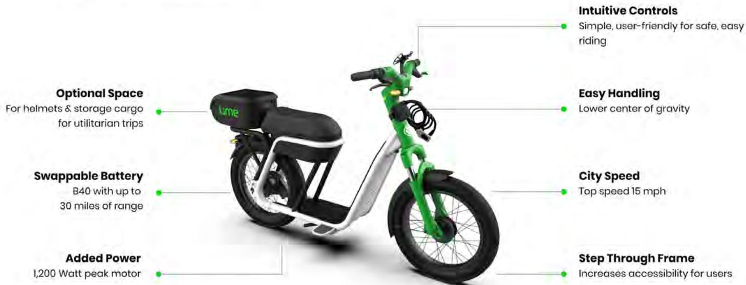
The Lime "Citra" is an all-electric seated scooter that gives riders all the benefits of three different vehicles — scooters, e-bikes, and mopeds — in one vehicle. Using Universal Design principles, Citra is designed to accommodate a wide range of individual preferences and abilities. Its intuitive controls are easy to understand, even for those with little experience with micromobility vehicles.
