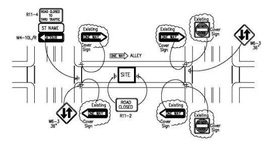
This plan shows how to change a One-Way Alley into a Temporary Two-Way Alley Maintain Local Access At All Times
