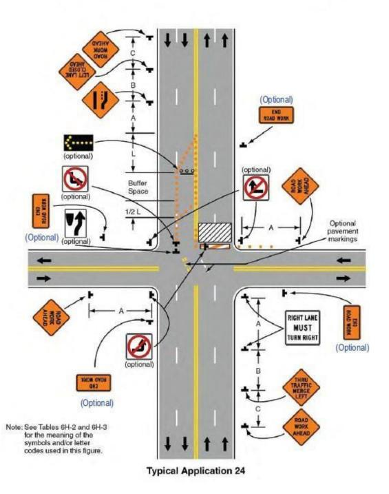
Figure 6H-25. Multiple Lane Closures at Intersection (TA-25)
