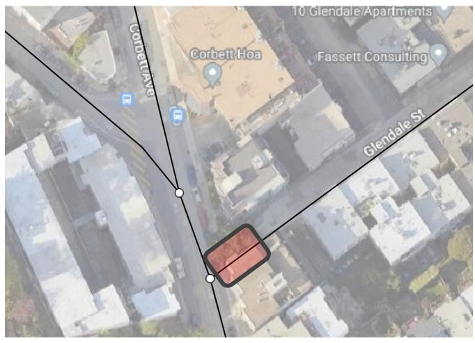
Figure 5: Example where network GIS data incorrectly represent two intersecting streets.
