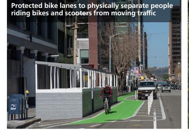
Travel lane reduction that encourages traveling at safer speeds and allocates space for other uses
