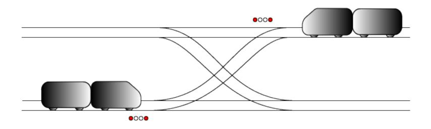
Need to control movement through junctions (called 'interlockings').
