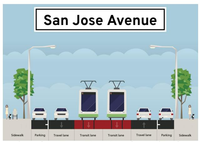
Figure 3: Proposed street cross-section on San Jose Avenue with new transit lanes. Left turns would also be allowed from the center (track) lane.
