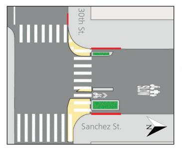
30th St. Gateway Treatment with potential island Painted Safety Zone at entryway of Sanchez Slow Street that includes a bicycle cutthrough and soft hit posts. Concrete islands with potential landscaping can be used to strengthen safety.
