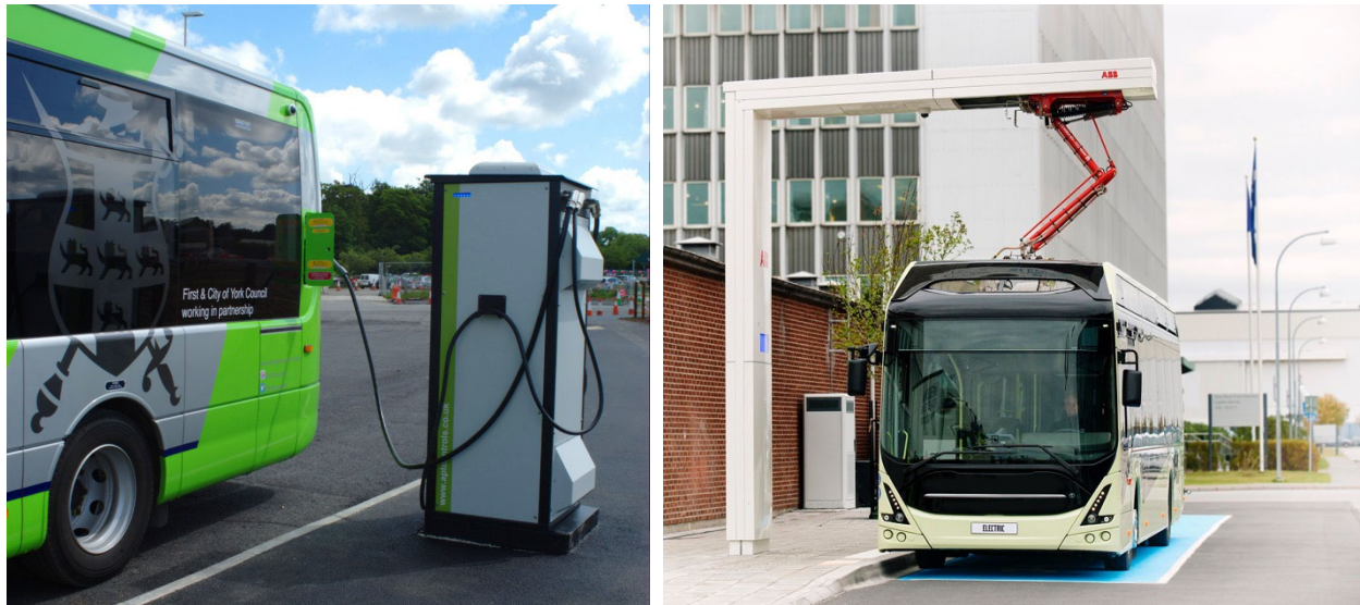
Figure 2-1. Plug-In and Pantograph Charging
