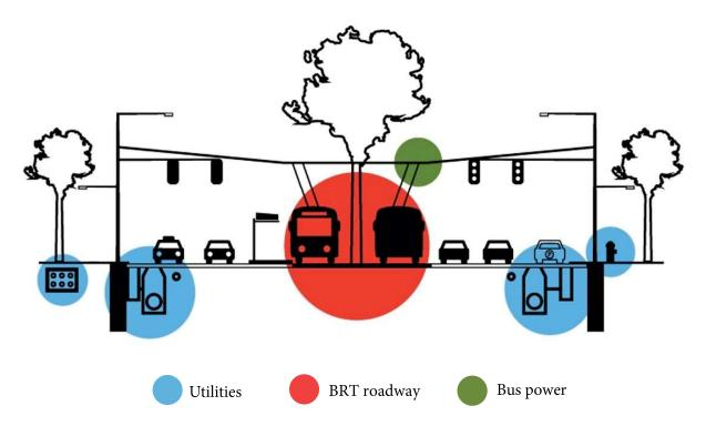
Figure 2. Overhead Contact System in a Center-Lane BRT Design<sup>9</sup>
