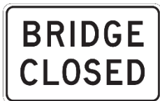
R11-2 (Alternate) Bridge
