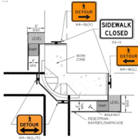
Figure 5.1b Pedestrian Detour at Intersection Corner (Non-Work Hours)
