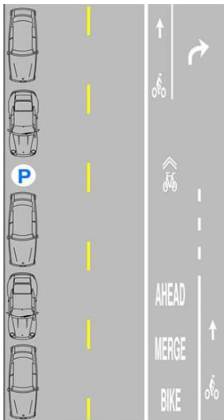
Fig. 9.1 Illustration of elements for shifting a bike lane to the left side of right turning vehicles
