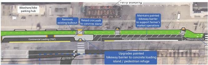
At both Clay Street and Don Chee/Ferry Building crosswalks, the project proposes to shorten the NB roadway crossing, straighten the bikeway and remove/replace traffic signal control with raised bikeway crossings and yield control. Triggers ADA upgrades across roadway, only marginal changes to existing curb uses.
