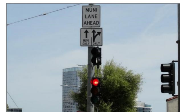
**Head start for buses on Haight Street at Buchanan Street:** This "queue jump" signal helps buses transition into a center bus lane from the curb. The vertical white bar (circled) is a special signal for buses, which get a head start to enter the intersection.
