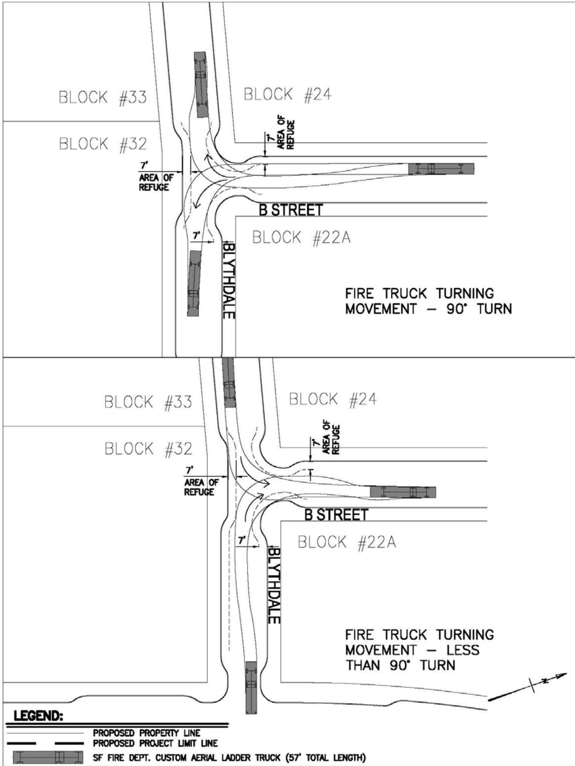
**SUNNYDALE HOPE SF** | FIGURE 7.15B ENLARGEMENT OF TYPICAL INTERSECTION FIRE TRUCK TURNING
