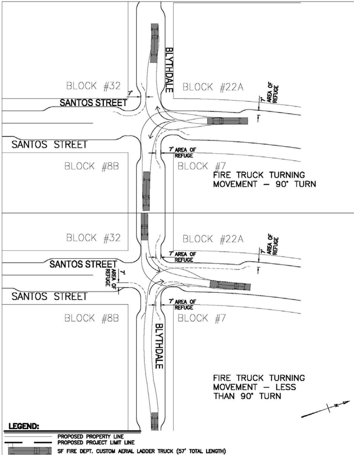
**SUNNYDALE HOPE SF** | FIGURE 7.15A ENLARGEMENT OF TYPICAL INTERSECTION FIRE TRUCK TURNING
